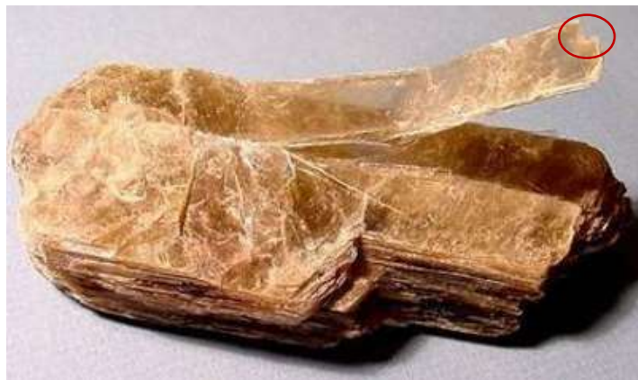
Figure 1. This mica has booklets that can be seen stacked on the front edge. In the back, one such elongated book has been peeled off and bent upward. On the very top left corner is also a fracture, where there is damage that is not a cleave (red circle.)
