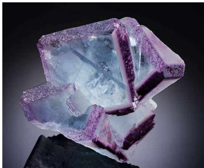
Figure 5. Fluorite with selective etching and selective color. The bevels are magenta and etched, while the cubic faces are blue and smooth. La Collada Mine, Asturias, Spain. Crystal Classics photo and specimen. (Also, can you see the cleave?)
